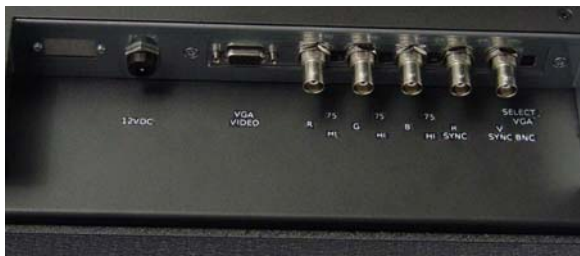
Video Input Interface with 5 BNC Input (RGB) option.
