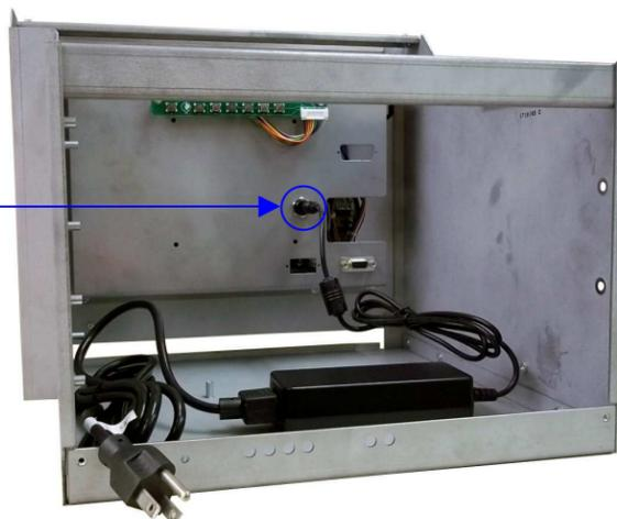
Plug Power Supply into Flat Panel Monitor.
