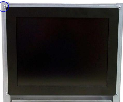
Mount Flat Panel Monitor to Chassis using screws from CRT mounting.
